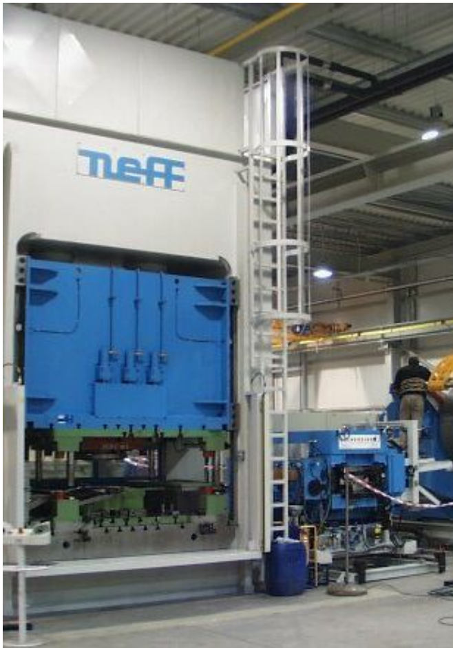
NEFF Double sided press DZP 400 with drawing cushion and tape feed
